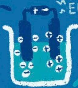
ELECTROLYSIS splits water into HYDROGEN and OXYGEN
